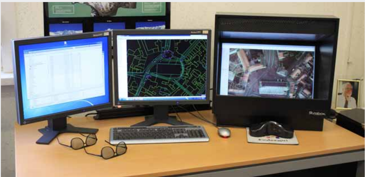
Photogrammetric production desk equipped with Orbit GIS, Strabo Photogrammetry Suite and 24" Strabox stereo viewing system.
